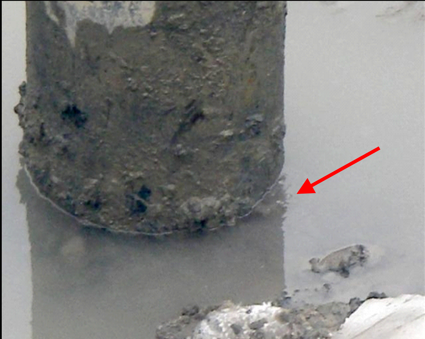
McLeod Oil Company Limited 00/15-03-020-03W5/0 Gas migration detected by presence of bubbles
